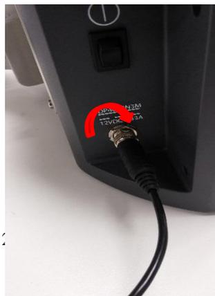
The power connector is classically plugged into the base. To prevent any accidental disconnection, you can lock the coupling screwing the nut on the base (from left to right, see picture above).
