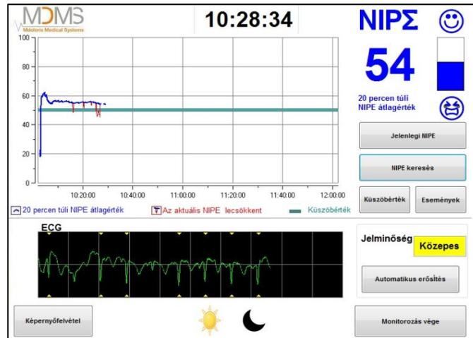
Figure 17 – Threshold value at the monitoring display
