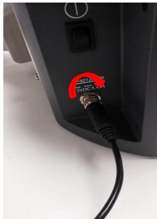
As usual, the power connector is plugged into the socket. To prevent any accidental disconnection, you can lock the coupling by screwing the nut on the base (from left to right, see picture above).
