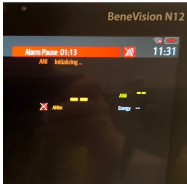
4. The ANI-MR module is now activated. This is verified when the ANI-MR parameters are displayed on the BeneVisionTM monitor.
