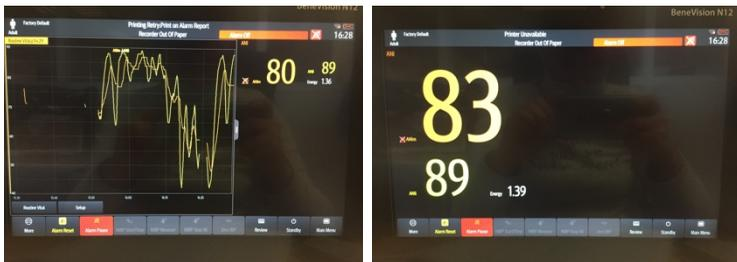
The ANI module window shows the information about the measurement acquired by ANI-MR. Three parameters are provided by the module:
